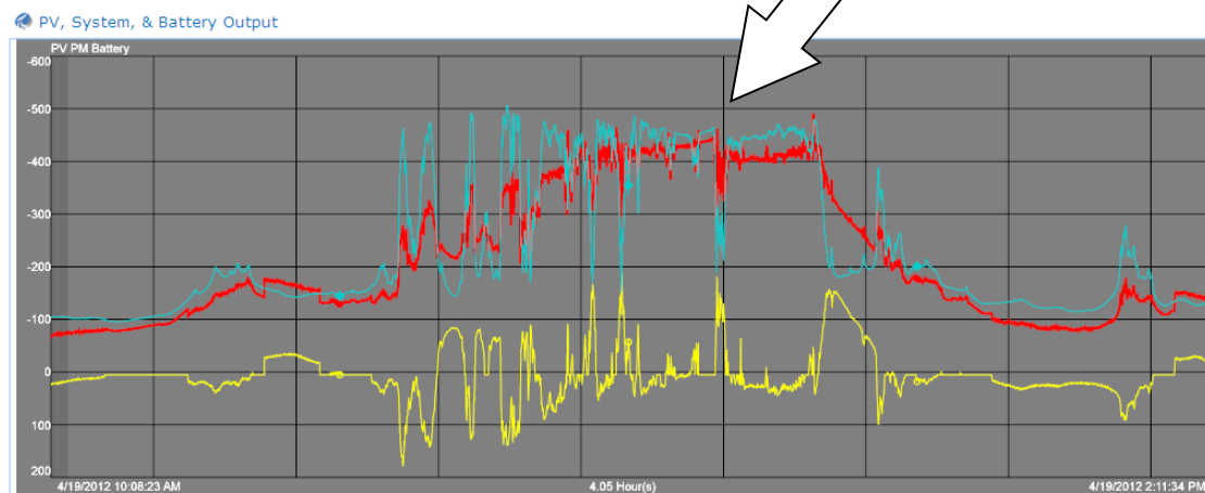
Figure 15 Magnified Smoothing with Irradiance Sensor Input
