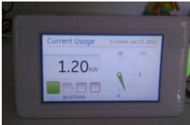
Figure 10.22. Example GE Home Energy Gateway Display 2
