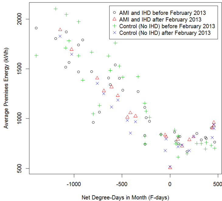
Figure 11.32. Measured Premises Energy Usage from Regression Models of the Test and Comparison Groups from Before and After February 2013 Plotted against the Net Degree-Days that Month
