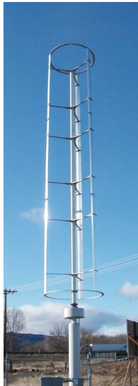
Figure 9.17. 1.2 kW Windspire Wind Turbine at the Ellensburg Renewable Energy Park (City of Ellensburg 2013a)
