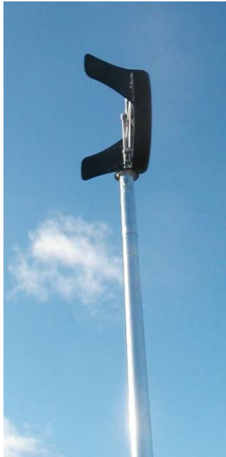
Figure 9.12. Residential-Class Honeywell 1.5 kW Turbine Installed at the Ellensburg Renewable Energy Park (City of Ellensburg 2013a)
