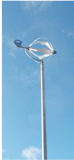
Figure 9.21. 2.25 kW Home Energy International Energy Ball V200 at the Ellensburg Renewable Energy Park (City of Ellensburg 2013a)
