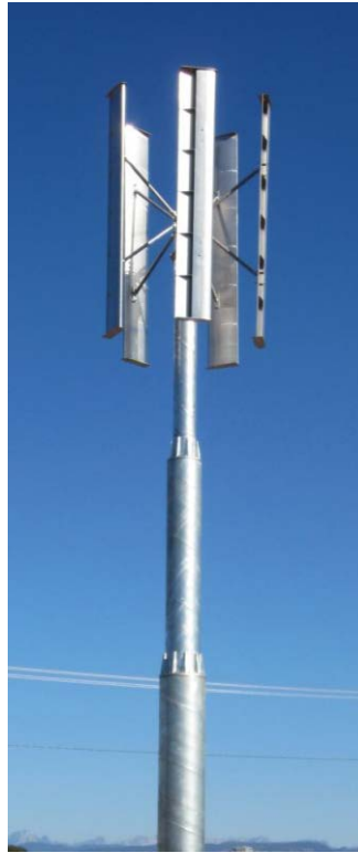
Figure 9.48. 1.4 kW Wing Power Wind System at the Ellensburg Renewable Energy Park (City of Ellensburg 2013a)
