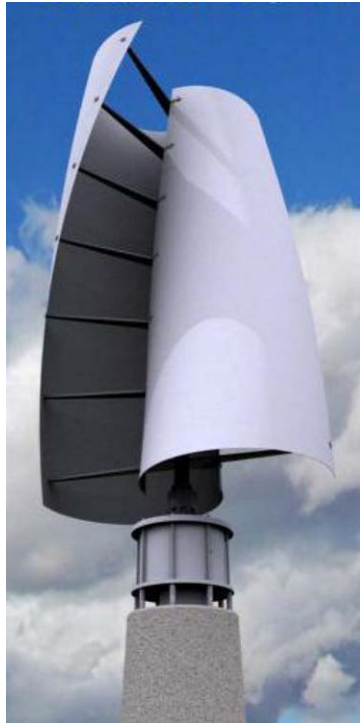
Figure 9.35. 10 kW Tangarie Wind System Installed at the Ellensburg Renewable Energy Park (City of Ellensburg 2013a)
