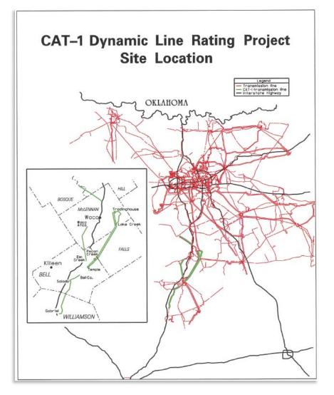
Figure 10 - DLR Project Area Showing Lines Selected for Instrumentation
