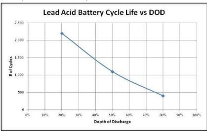
Figure 6. Lead Acid Battery Cycle vs. DOD
