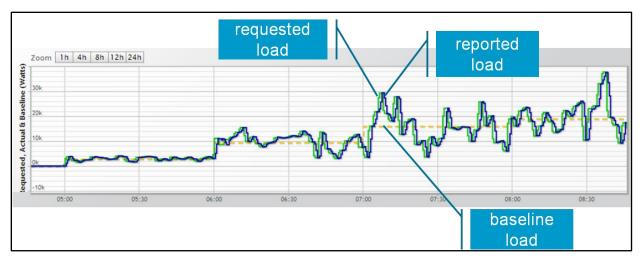
Figure 10. Near Coincidence of Requested vs. Reported Load from GETS System Aggregated Group in Response to Simulated ACE Signals for Frequency Regulation
