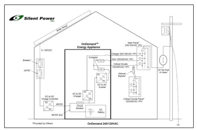
Figure 1. Simplified SP Installation Wiring Diagram
