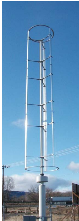
Figure 9.17. 1.2 kW Windspire Wind Turbine at the Ellensburg Renewable Energy Park (City of Ellensburg 2013a)
