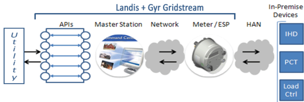
Figure 2-25: Communication Flow from the AHE to the HAN via the FAN
