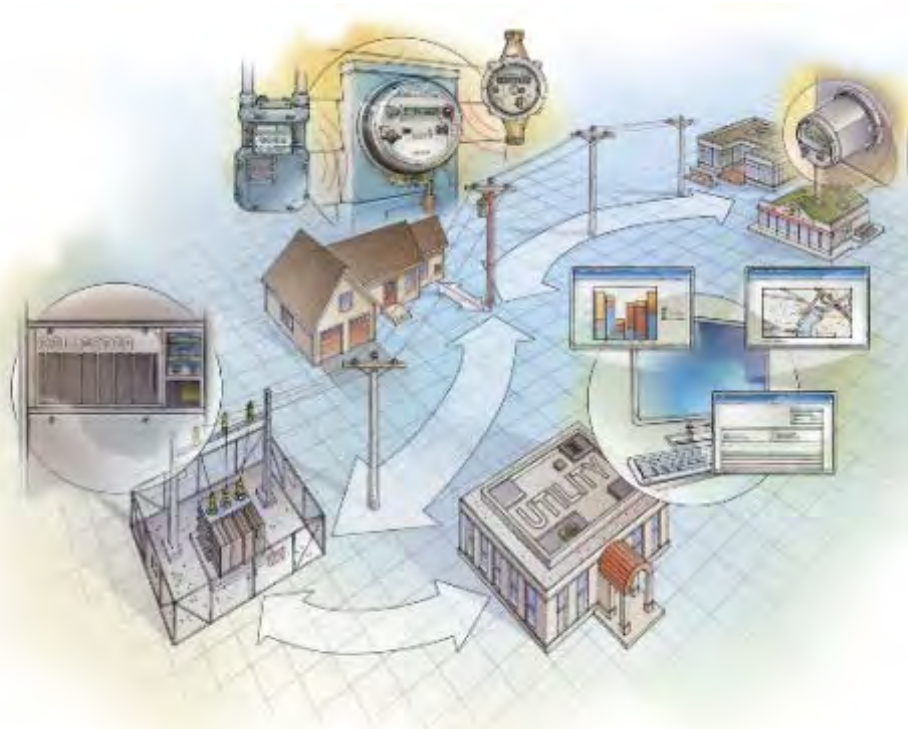
Figure 2-24: AMI RF Mesh FAN
