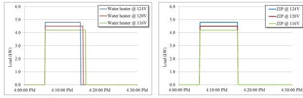
Figure 6. Comparison of Physical Water Heater Model versus Zip Model at Three Voltage Levels
