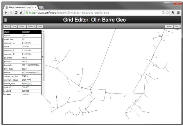
Figure 3. Specifying Capacitor Bank Properties in the OMF
