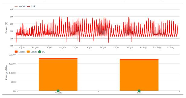
Figure 5. Three-Month Dynamic Powerflow Simulation—Powerflow across the Substation, and Loads and Losses Breakdown
