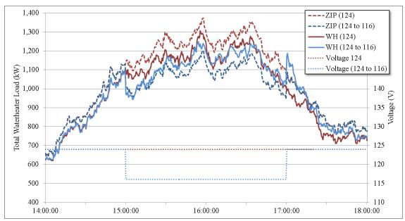
Figure 7. Peak Reduction Event-Shifting Voltage from 124 to 116 and Comparing Physical Water Heater Load vs. ZIP Load
