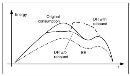
Figure 1. Impact on Demand over Time and Difference between DSM and EE Measures
