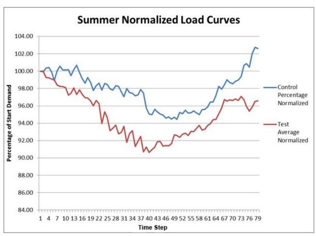
Figure 3. Averages of Test and Control Data over Test Period, Summer
