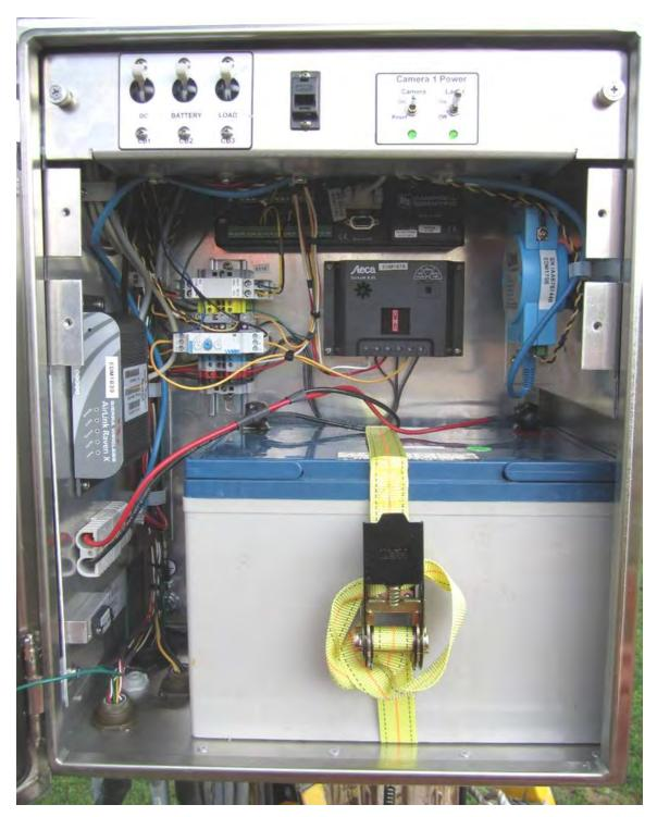
Figure C-21 Sagometer electronics box
