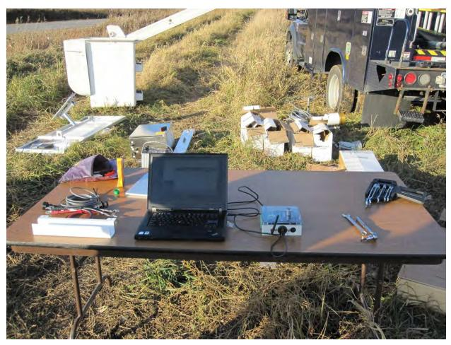
Figure C-43 Remote ZAP Unit used to check communications of the EPRI Sensors in the field
