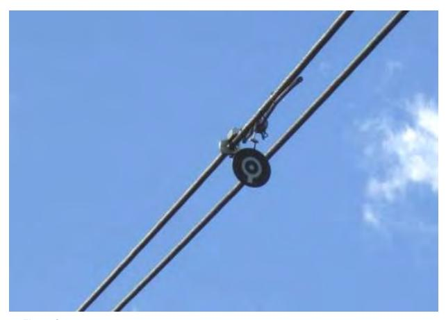
Figure C-37 Sagometer target
