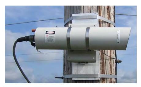
Figure 3-2 The sagometer camera
