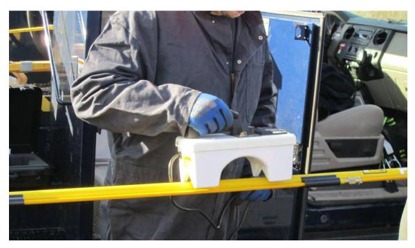
Figure C-41 Lineman tests hot stick prior to installing the EPRI Sensors on the energized 230 kV line
