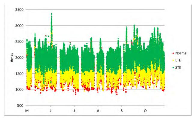
Figure F-51 Overhead line ratings based on the Sagometer at Site 1 – Summer 2011
