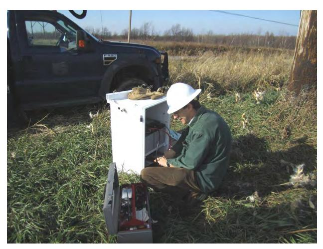
Figure C-47 ThermalRate Battery Box Being Wired
