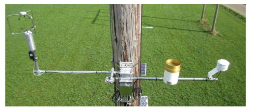
Figure 3-1 Weather station sensor array; anemometer, pyranometer, rain gauge, temperature/humidity sensor (left to right)
