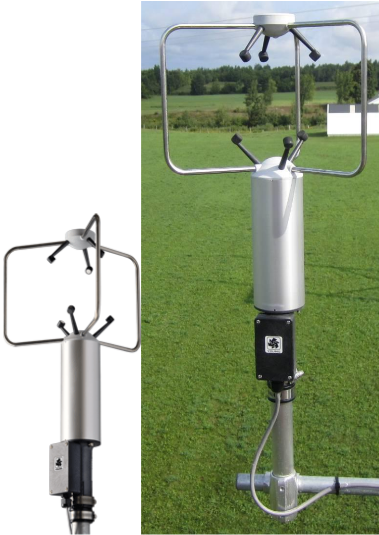
Figure 3-10 3 axis wind speed and direction sensor. Note the wire junction box should always point south. This keeps the wind direction aligned to a known compass heading.
