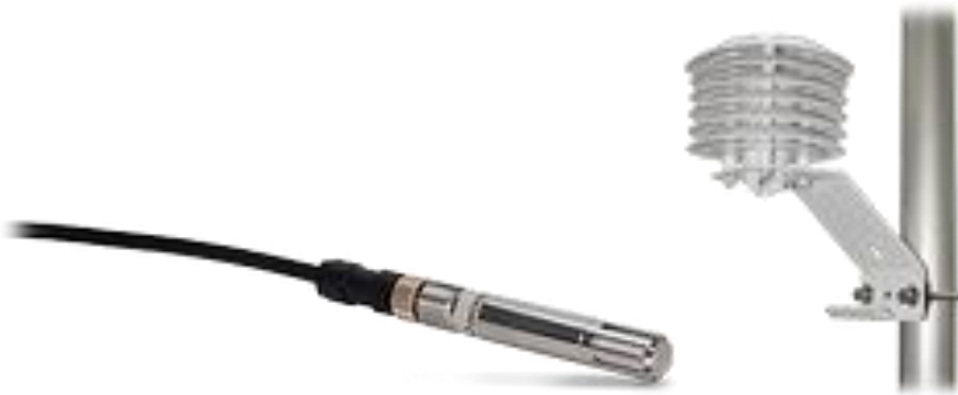
Figure 3-2 Temperature sensor removed from housing, housing shown to the right of the sensor
