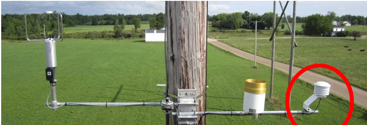
Figure 3-3 Weather station array highlighting the humidity sensor
