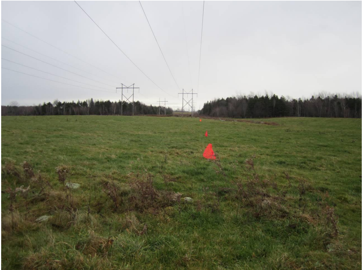
Figure 4-36 Locations were marked under the line for the Sagometer target and EPRI sensors
