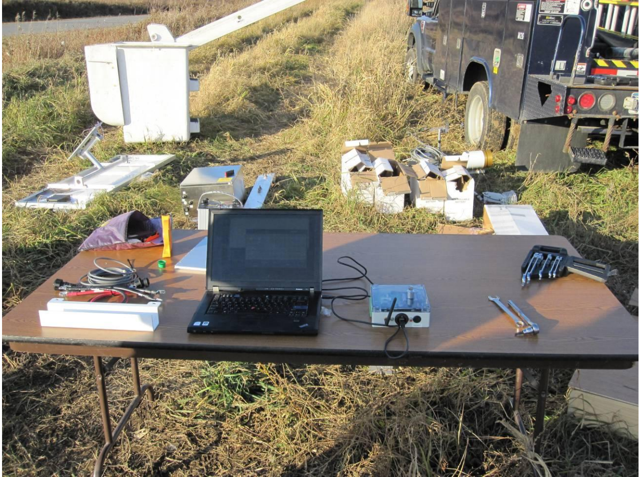
Figure 4-22 Remote ZAP unit used to check communications of the EPRI sensors in the field
