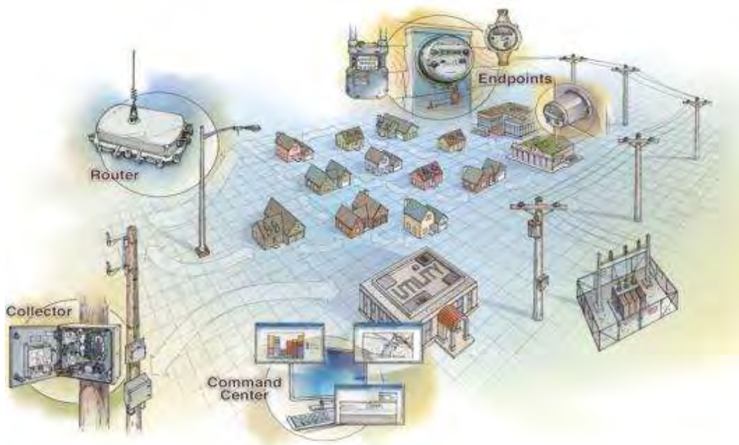
Figure 2-18: L+G Gridstream AMI Command Center and FAN
