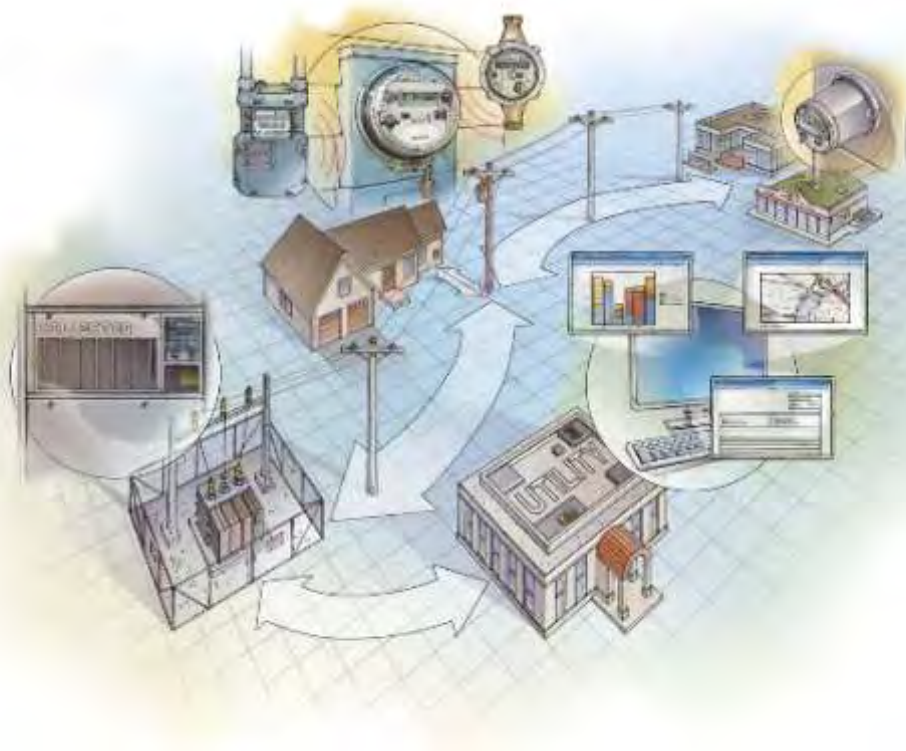
Figure 1-7: AMI RF Mesh FAN
