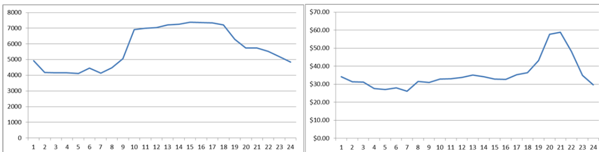
Figure 4.7: Sample hourly load (kW) and real time price ($/MWh) of the IIT Microgrid (winter weekday)
