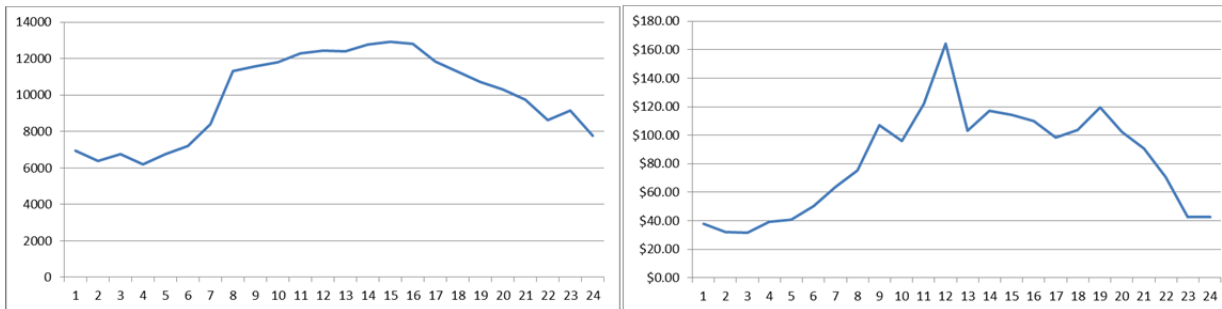
Figure 4.6: Sample hourly load (kW) and real time price ($/MWh) of the IIT Microgrid (summer weekday)
