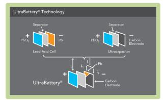
Figure 3. Lead-acid cell (top left), ultracapacitor (top right), UltraBattery<sup>®</sup> (bottom). Courtesy of East Penn.
