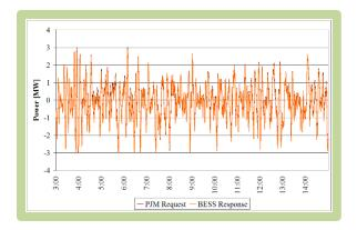
Figure 2. BESS response to 3 MW PJM Regulation Signal
