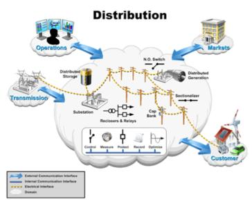
Figure 3 - NIST Smart Grid Conceptual Distribution Domain
