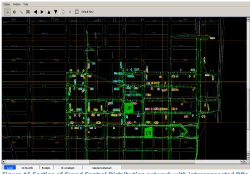
Figure 16 Section of Grand Central Distribution network with interconnected DRs
