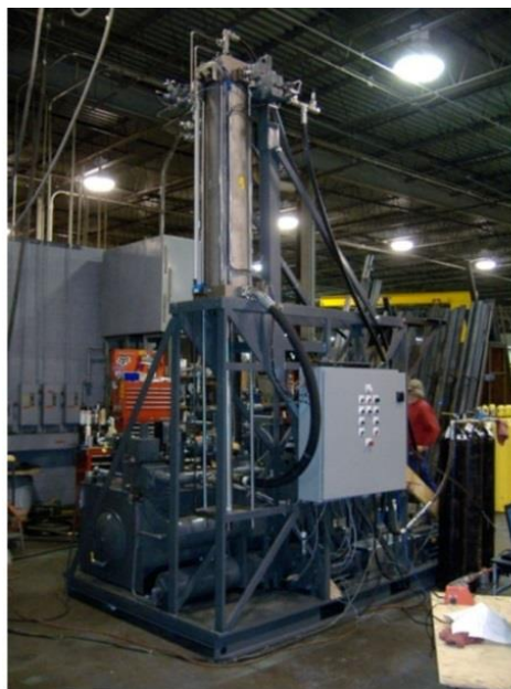
Figure 6: Left: Heat-transfer test stand, a.k.a. HXTST. Right: Experimental results for an isothermal expansion (red) vs. adiabatic expansion (blue) vs ideal expansion (black) for the same mass of air. Dots are marked at 1 second intervals for reference. Grey lines are lines of constant temperature at 25°C increments from ambient temperature.
