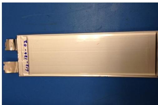
Large Format Cell 1 Capacity: ~2 Ah Size: 72 x 234 x 2 mm
