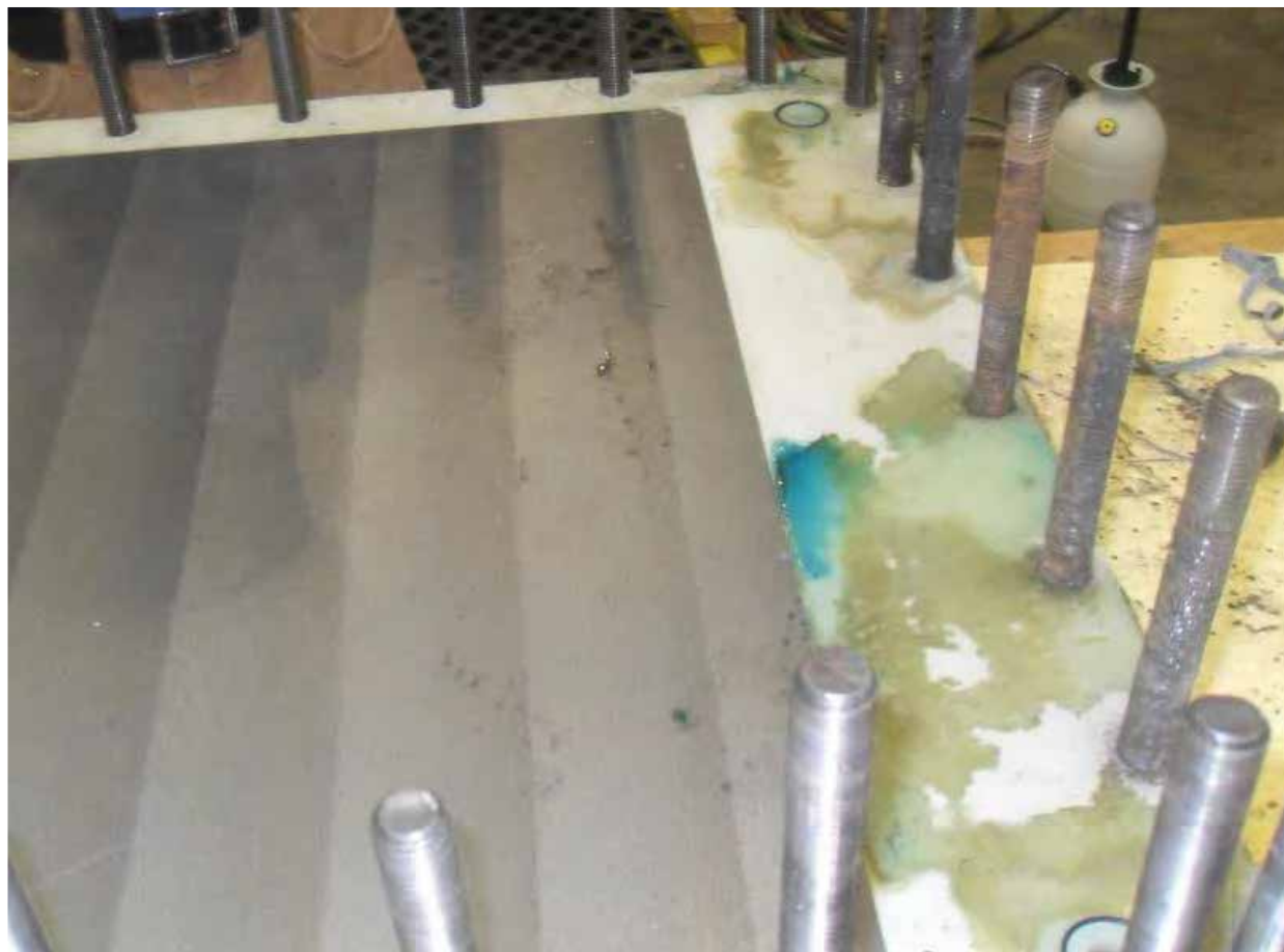
Figure 31 Prototype 8 Top Cell Disassembly Showing Pooling of Electrolyte
