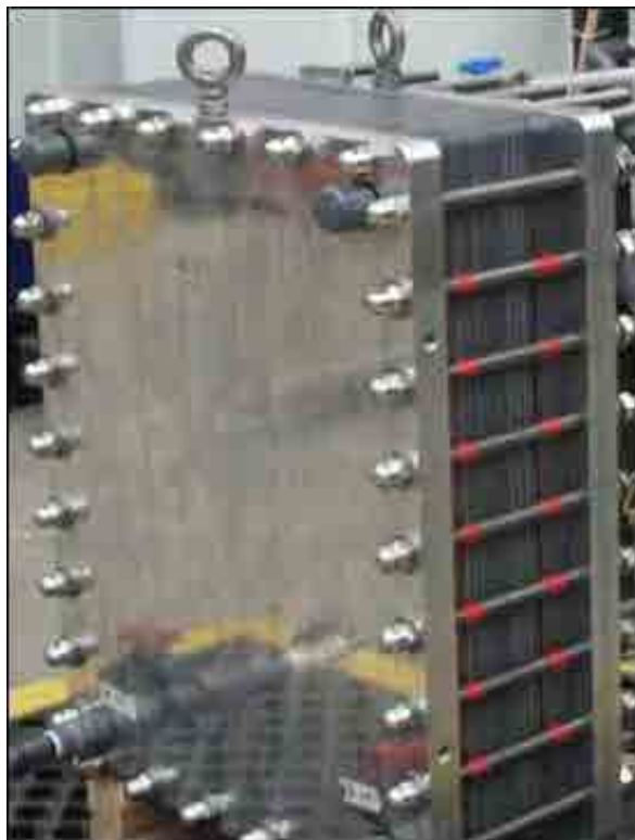
Figure 27 Photograph of a 2.5 kW, 10 cell stack.
