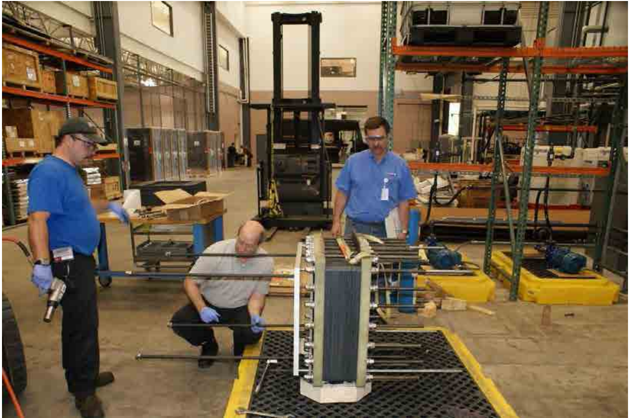
Figure 30 Large 10 kW stack (Prototype 8) being installed at CTC for testing.
