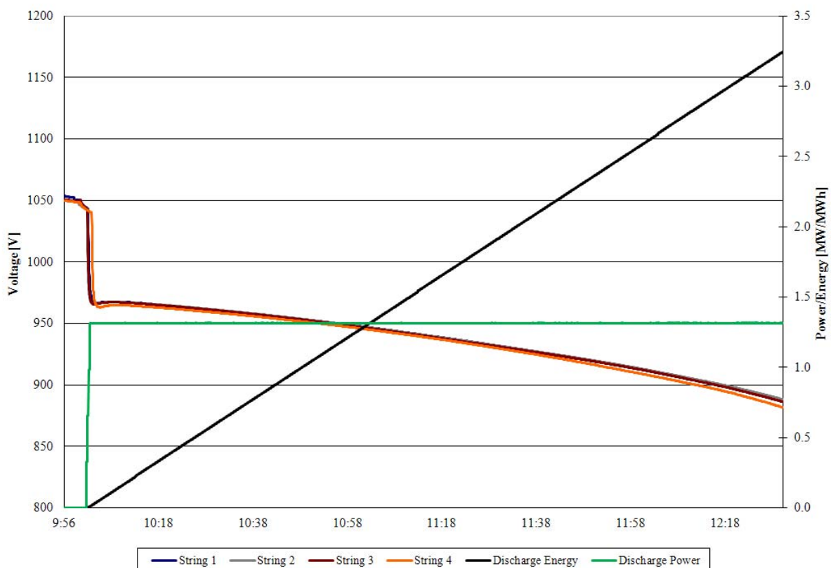
Figure 7. Power, energy, and string voltages during capacity discharge.
