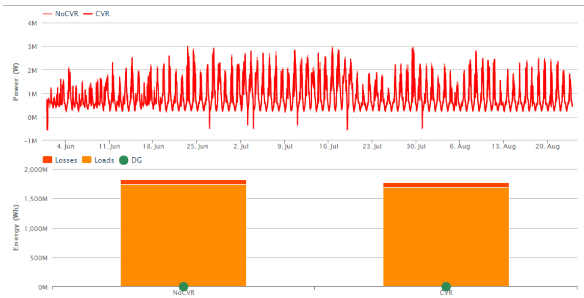
Figure 9.5: Three-Month Dynamic Powerflow Simulation—Powerflow across the Substation, and Loads and Losses Breakdown
